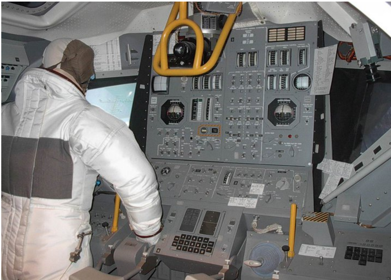
10 - This is the inside of the Lunar Module, and you can see the AGC DSKY in the lower center near the astronaut's right hand, again placed close to the center of the landing module so that either astronaut could easily access the controls.
