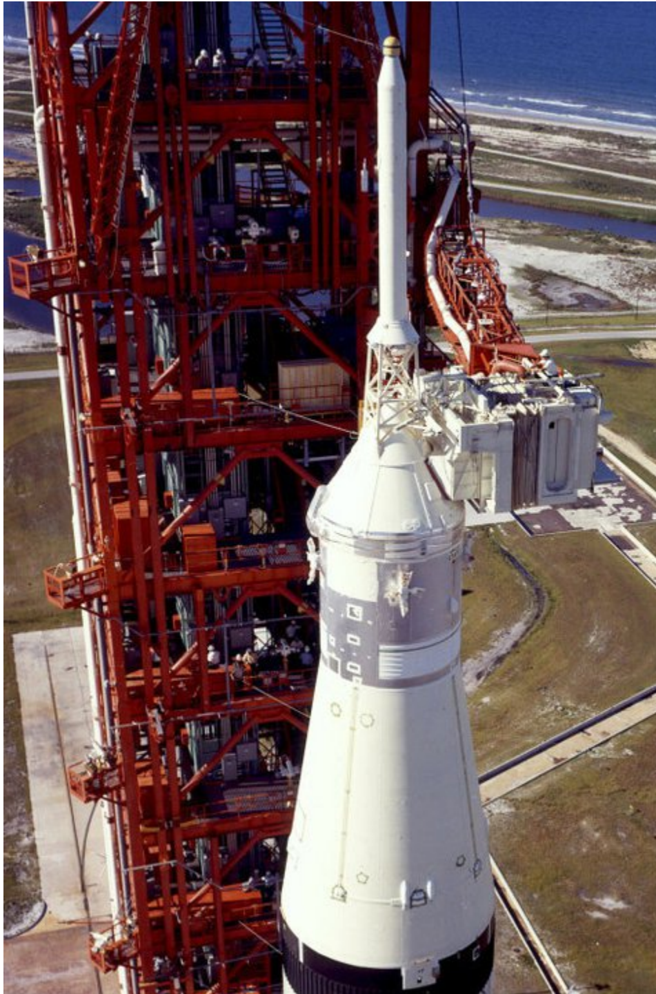
14 - On July 11, 1969, the Saturn V is on the launch pad and is being prepared for launch. In this photo, you can see the top section of the Command Module (CM), just below it is the Service Module (SM), and in the tapered section below SM is the enclosed Lunar Module (LM). The white boxy structure attached near the top of the Command Module is what I recall as the 'White Room' and it provides the sheltered entry point into the CM for the astronauts. The astronauts first take an elevator to the attachment level, walk down the connecting bridge, and finally climb into the CM.
