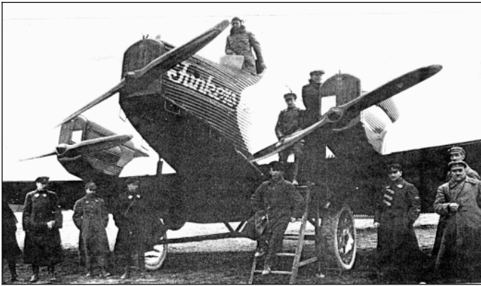
Junkers built the first all metal, trimotor bomber of the Red Air Force, shown here at a Russian airport in 1926.
