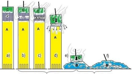
I. Crush-Down Phase II. Crush-Up Phase http://www.nistreview.org/WTC-PROGRESSIVE-COLLAPSE-BAZANT.pdf
